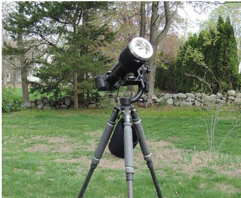
Fig. 13 The camera, telephoto lens, mount and solar filter covering the objective lens are shown
